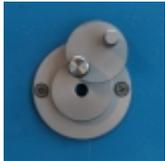
Thermocouple connector (installed in the door of the furnace, acid-proof frame, max diameter 11mm).
