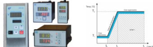
Two four character displays allow easy reading of the actual temperature of the object and set parameters. With the ability to program a delayed start time as well as the holding time, i.e. to maintain furnace temperature for a certain time, it is possible to automatically carry out a series of burnings unattended. This gives you the opportunity to work eg. during the night tariff for electricity or to heat-up the furnace to the required temperature ahead of time, avoiding unnecessary downtime.
