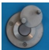
Sight glass installed in the door of the furnace. Diameter 20 mm.
